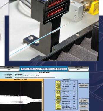
The MSI FFS760S PTCA Balloon Catheter Pleating and Folding Equipment doubles machine output through the use of dual in-line Wavepleat<sup>™</sup> and fold heads. This machine allows for processing on one set of heads while the other set is being loaded, effectively allowing a single operator to simultaneously control two machines. Integrated vision systems eliminate manual positioning variability and associated yield loss by automatically positioning balloons into the pleat/fold heads.
