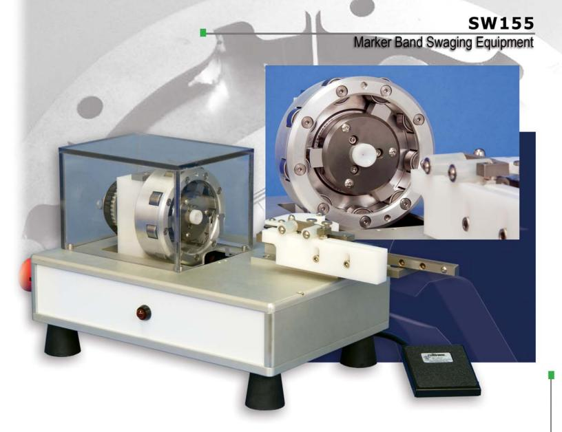
The MSI SW155 utilizes our proprietary, robust, Element™ swaging technology and is intended for use in swaging metal bands of a wide range of materials.
