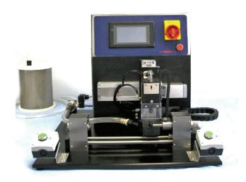
**PlasticWeld's HPD-6** table-top fully programmable drilling system with slug ejection and capture. This single spindle drill places holes along a 6 inch segment and the program allows virtually unlimited number of holes with varying spacing and rotation. Designed for maximum flexibility for clean room use.
