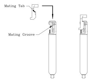
Figure 3.11 Installation of Ground Jaw onto RF Jaw/Tube Assembly
