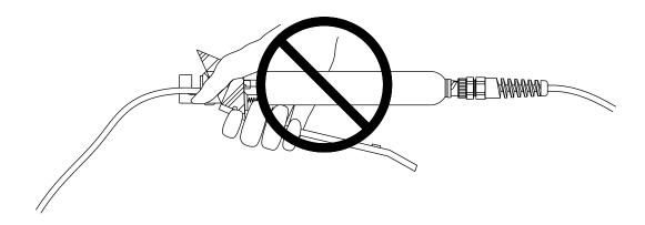
Figure 2.5 Incorrect Technique for Holding the Sealing Head
