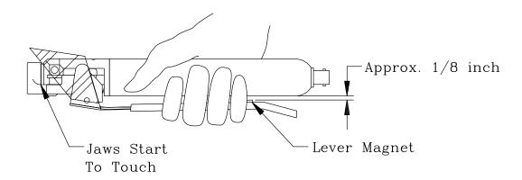
Figure 3.2 Correct Lever/Sealing Body Gap
