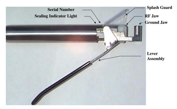
Figure 1.1 Model 4105 Hand Held Sealing Head
