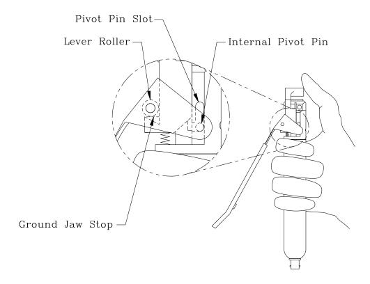
Figure 3.13 Installation of Lever into Pivot Slots
