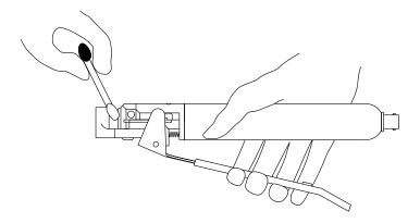
Figure 3.4 Drying the Sealing Region
