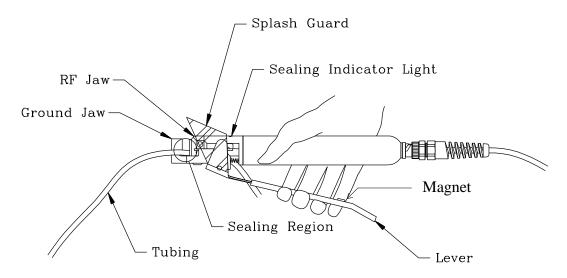
Figure 2.4 Correct Technique for Holding the Sealing Head
