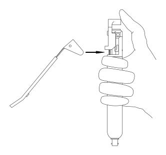
Figure 3.12 Installation of Lever on to Sealing Head
