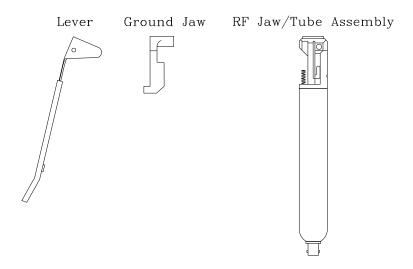
**Figure 3.9 Sealing Head Components**
