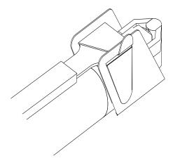
Figure 2.2 Splash Guard Tab
