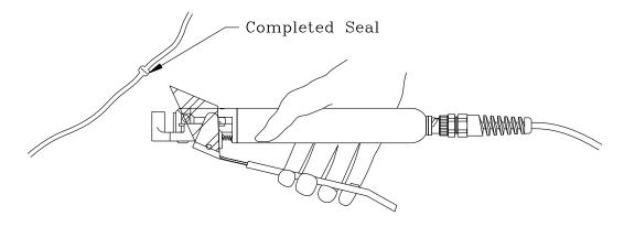
Figure 2.7 Releasing the Sealing Head Lever at Seal Completion
