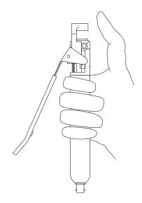
Figure 3.14 Final Assembly of Sealing Head
