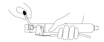
Figure 3.6 Drying Ground and RF Jaw Surfaces
