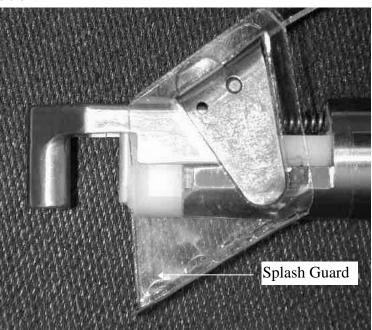
Figure 2.3 Final Attachment of Splash Guard
