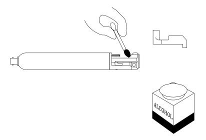
Figure 3.10 Cleaning Individual Sealing Head Components
