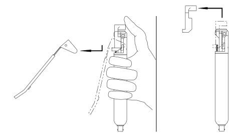
Figure 3.8 Removing the Lever and Ground Jaw
