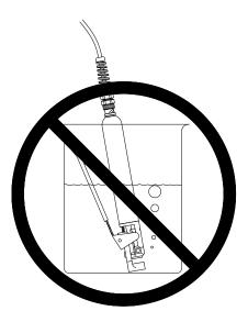
Figure 3.1 Incorrect Cleaning Technique
