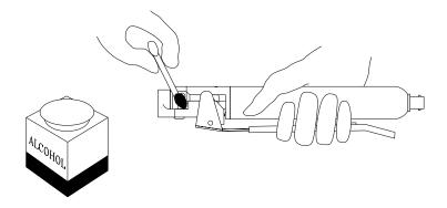
Figure 3.5 Cleaning Ground and RF Jaw Surfaces
