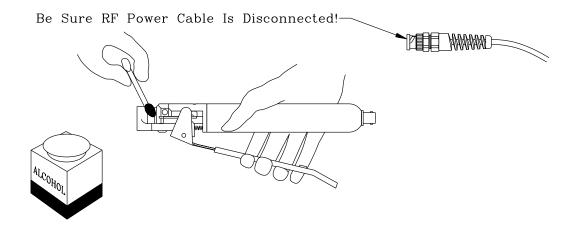
Figure 3.3 Cleaning the Sealing Region
