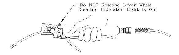
Figure 2.6 Maintaining Compression During the Entire Sealing Process
