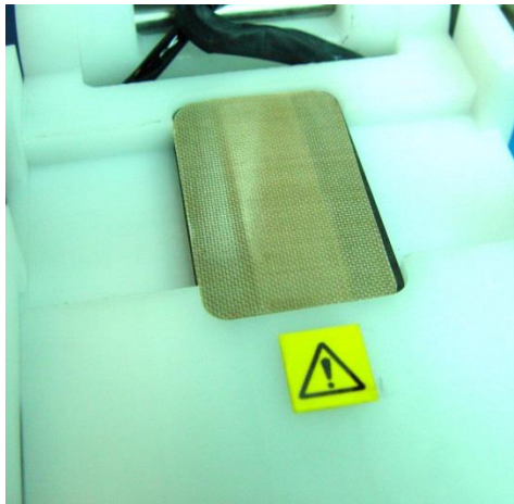
Figure 2.9 Teflon fiberglass adhesive barrier application
