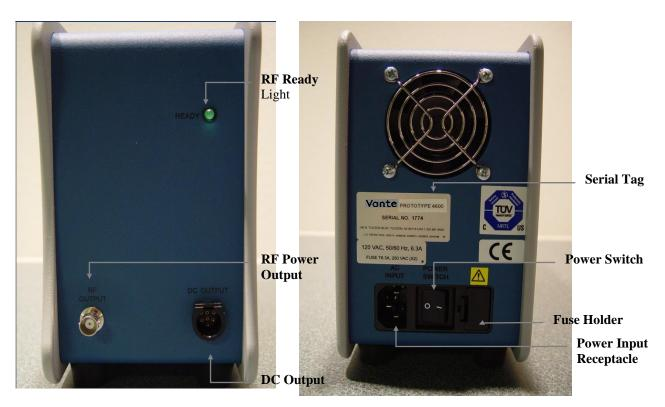
Figure 1.3 RF Power Source Power Interface Panel
