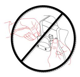
Figure 2.8 Incorrect Sealing Method
