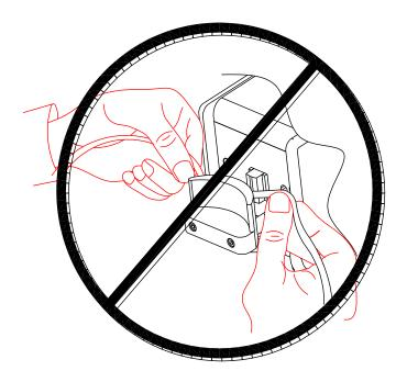
**Figure 2.2 Incorrect Technique for Holding the Tubing**
