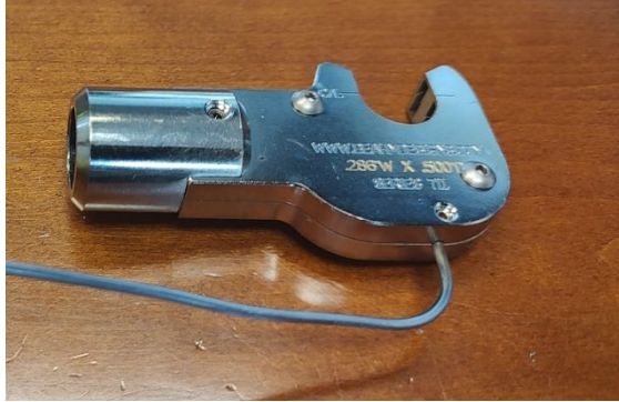
Figure 3. Secure thermocouple wire placement
