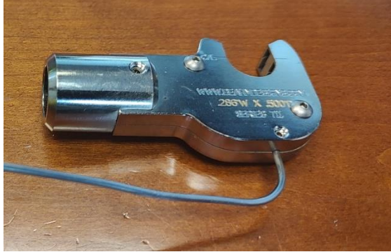
Figure 8. Secure thermocouple wire placement
