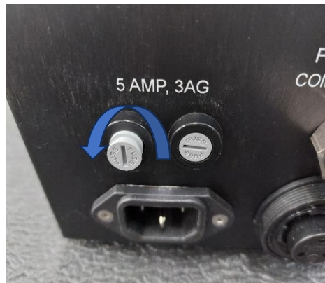
Figure 9. Removing Fuse Insert
