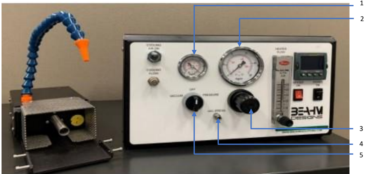
Figure 3. Balloon Development System (Model 210-A)
