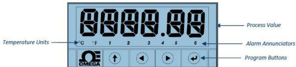
**Figure 4. Controller Layout**
