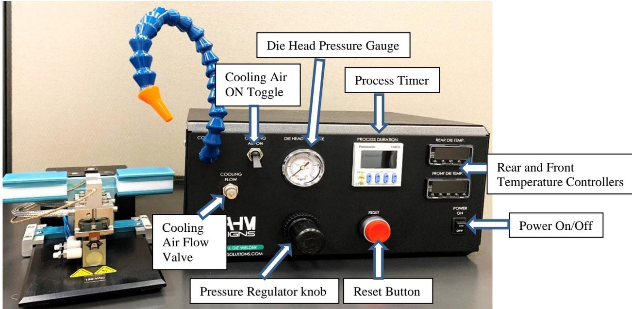
Figure 1. 220-B Split Die Thermal Bonder Front Panel
