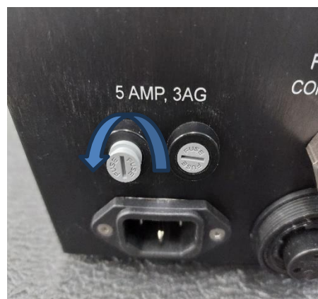
Figure 3. Removing Fuse Insert
