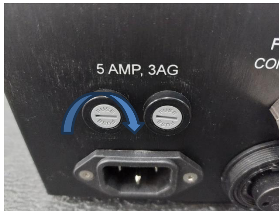
Figure 5. Fuse Insert Replacement
