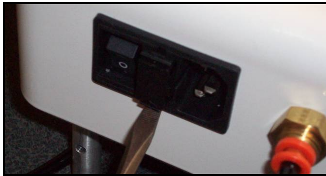
Figure 3.1 Fuse Holder Release
