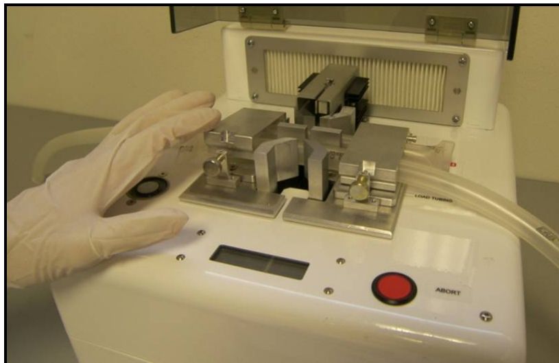
Figure 2.5 Closing clamps to secure tubing
