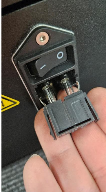
Figure 46. Power Entry Module Fuses
