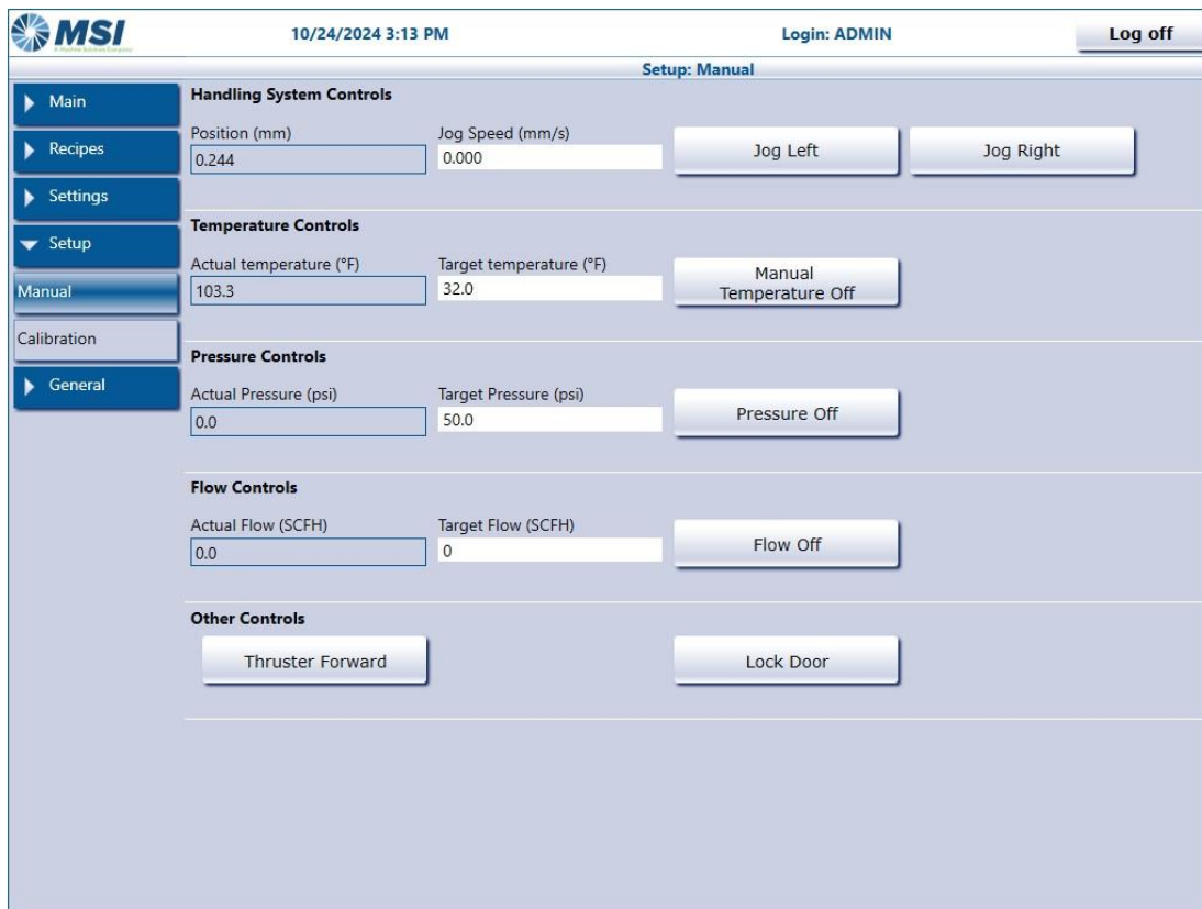
Figure 31. Manual – Controls screen
