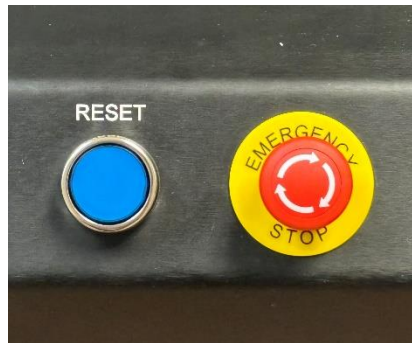
Figure 3. E-Stop and Reset
