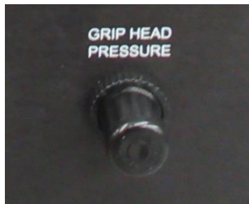
Figure 6. Grip Head Pressure Regulator
