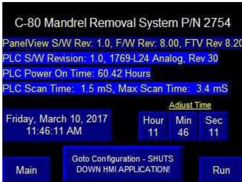
Figure 17. PLC Status and HMI Shutdown Screen Buttons/Displays and Descriptions
