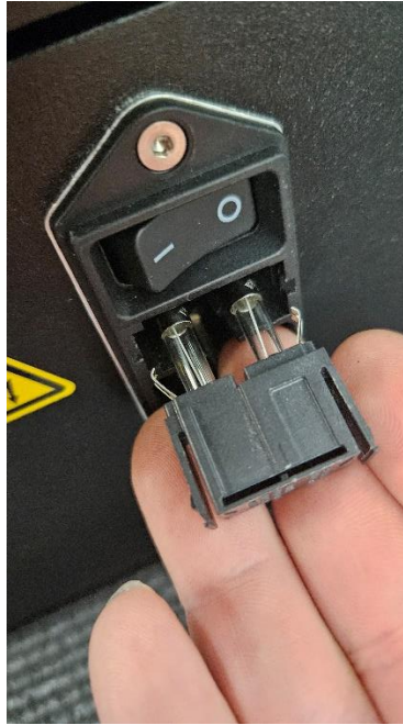
Figure 5. Power Entry Module Fuses
